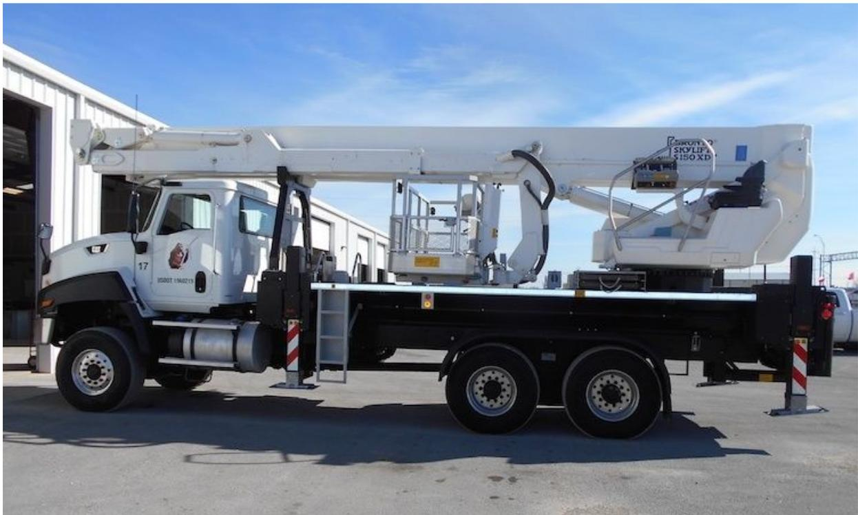
Some features of this model include robust Cat chassis, auto-leveling outriggers, 360° continuous rotation, a working platform of 3 ft x 7 ft with a basket capacity of 1,500 lbs, voice-in-command intercom, integrated in-basket water/electricity/air, and more.
